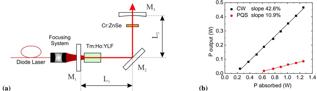
Fig. 1. (a) Setup of the PQS Tm,Ho:YLF laser. M<sub>1</sub>: dichroic pump mirror, M<sub>2</sub>: HR-laser, HT-pump mirror, M<sub>3</sub>: output coupler. (b) Output power vs. absorbed pump power for 5.8% OC in CW and PQS regimes.
